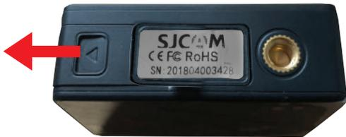
Open the battery cover by sliding it to the side. The battery cover will spring outward.
