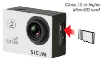
Insert a MicroSD card as shown in the illustration above, with the label facing the LCD screen, until it clicks into place. To remove, just push it in gently and the card will eject. **NOTE:** To make sure you do not lose any data, only remove or insert your card while the camera is off.
