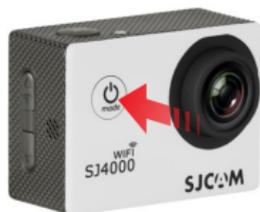
Press the Power/Mode button to turn your camera on. You will hear a beep, indicator LEDs will light up, and the screen will display the SJCAM logo. Default Mode is Video. To turn off your camera, long-press the Power/Mode button.
